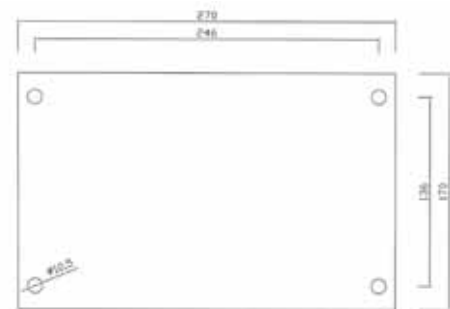
Drawing top- and bottom plate Thickness 8 mm.
